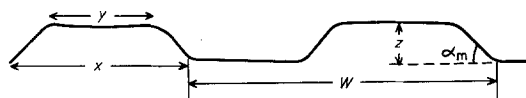
Figure 3 Cross-section of a photoresist etched silica substrate defining parameters whose dimensions are quoted in Tables IA and B.
