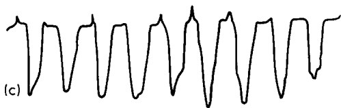
Figure 7 Structure of deeply photoresist etched silica surface as revealed by (a) and (b) scanning electron microscopy ( \times 42 ) and ( \times 164 ) and (c) surface profilometry ( \times 3100 vertical) and ( \times 124 horizontal).
